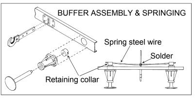
snip off some of the narrow end of the shank to leave just over 1mm from the step, and solder a retaining collar onto the shank. Open up holes in buffer beam slightly and fit buffers.
