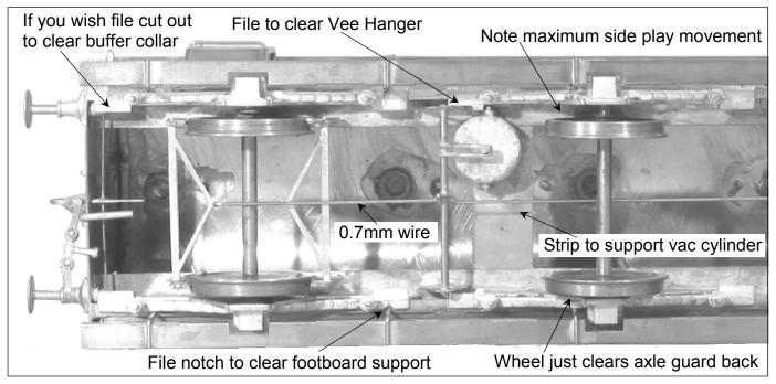
The above illustration shows the underside of the brake 3rd coach but the all 3rd is the same with the exception that the second vee hanger is fitted to a wider rectangular strip 2/3 of the way across the coach and the brass rod is correspondingly shorter.
