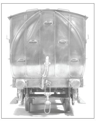
down again and run fillets of solder up the inside of the joints. Again work 1/3 at a time on alternative sides (watch out for the ends bowing inwards with the heat) and then repeat for the stepped end. Then dress the outside of the joints to give crisp square corners.
